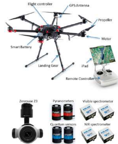
Figure 4.1: example of a remote-sensing vehicle: The DJI's Matrice 600 for Measuring Land Surface Albedo [400]
