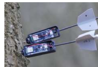
Figure 4.4: Impulsive launching of sensors to monitor the health of forests [345]
