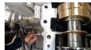
Figure 4.44: A conventional vibration probe tip is pressed against a surface by hand.
