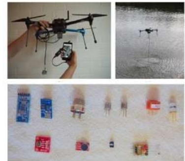
Figure 4.3: A low-cost, open-source, modular sensor platform [341].
