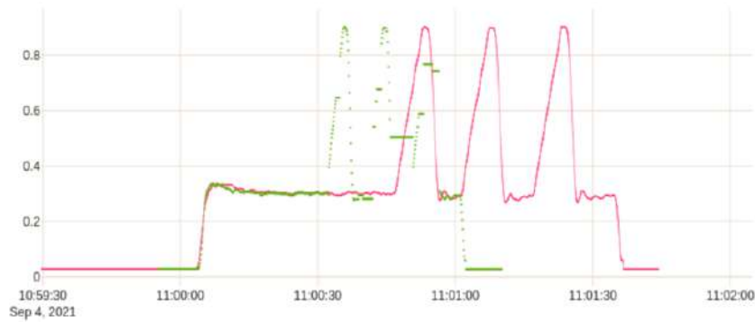
Figure 3.46: Pose Latency Graphs: Z position of Drone over time, for avatar (green) and real drone (red).
