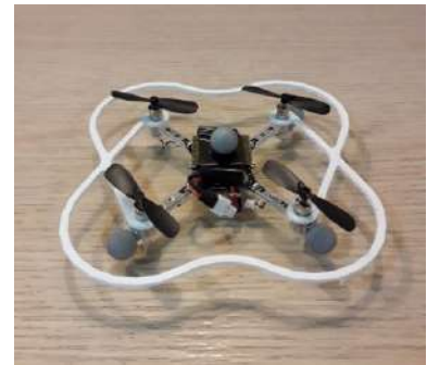
Figure 2.5: The Crazyflie 2.1 miniature quadcopter with four motion-capture markers, expansion boards (not visible), and battery.
