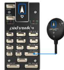
Figure 4.11: The Pixhawk4 and GPS: an advanced autopilot adopted by academic and commercial developers [403].
