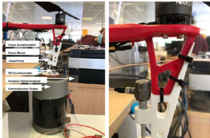
Figure 4.46: Installation of External Accelerometer
